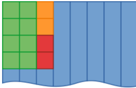
Figure 3.6: Conflicting accesses in the same memory partition (vertical stripes)
