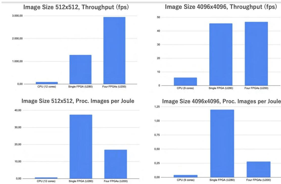
Figure 110: [FIPLib] CPU, Single- and Multi-FPGA implementation performances comparison
