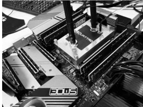
Fig.1.5.1.3 Testing Two-Phase Cooling System on AMD Threadripper 3990X at 3DWS Laboratory
