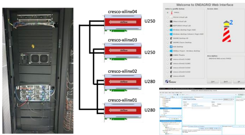
Fig.1.4.1.9: The ENEA FPGA Lab, with F.A.R.O as GUI to develop with VITIS and Intel OneAPI
