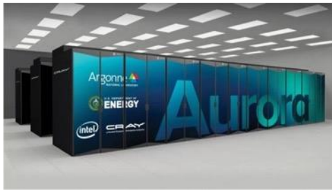
Fig.1.4.1.2: Aurora: a 2 ExaFlops peak performance supercomputer with Intel Pontevecchio XE-HPC GPUs
