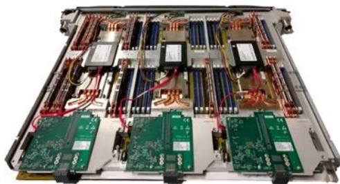
Fig.1.5.2.2a: Bull Sequana compute blade with three compute nodes
